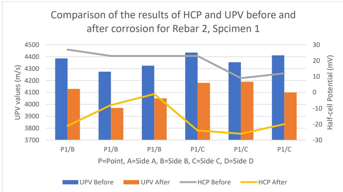
Figure 10: The Comparison of the results of HCP and UPV before and after corrosion for Rebar2, Specimen 1
