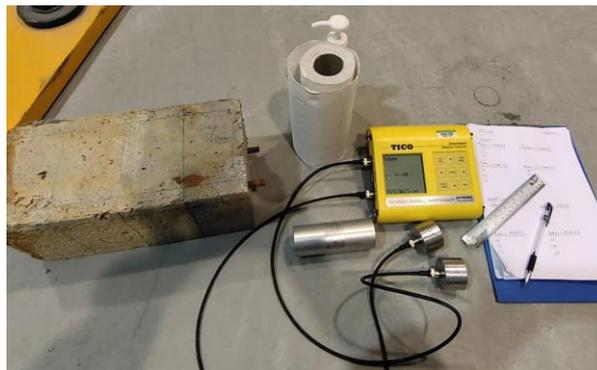
**Figure 8: Preceq Tico Ultrasonic Instrument used**
