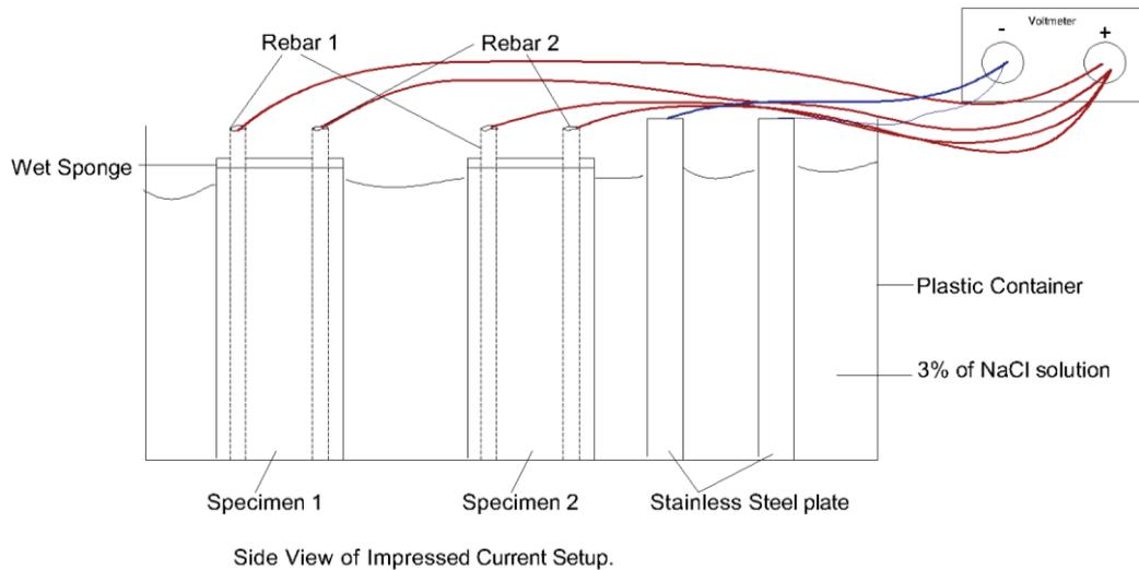
**Figure 4: Setup of Impressed Current test for the project**
