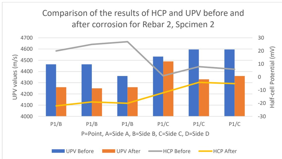
**Figure 12: The Comparison of the results of HCP and UPV before and after corrosion for Rebar2, Specimen 2**
