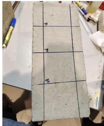
**Figure 6: Mark out location of the specimen**
