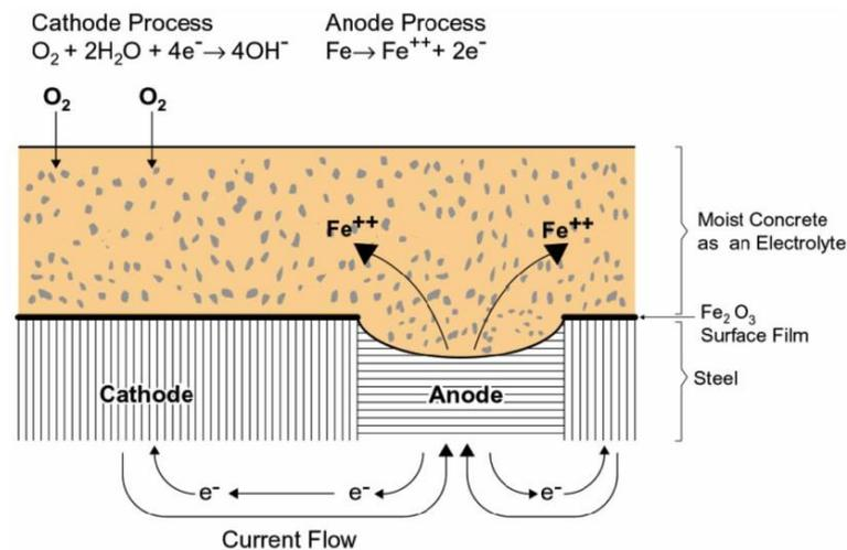
Figure 1: The electrochemical process [7]
