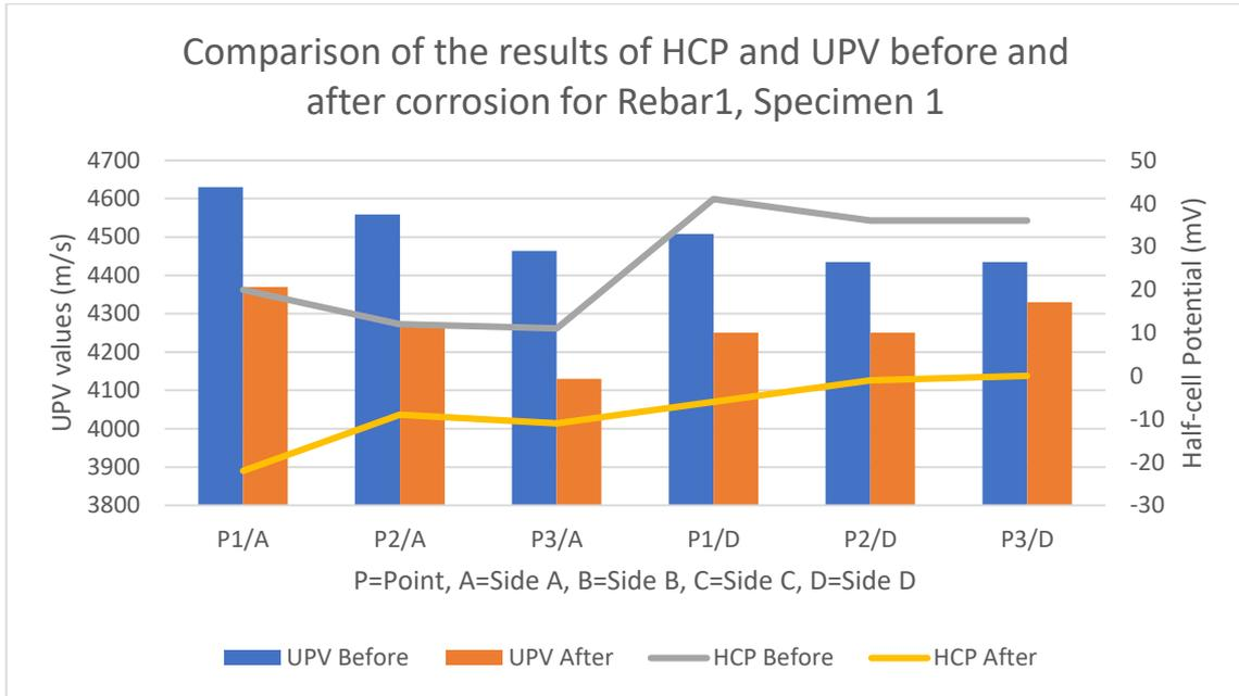
Figure 9: The Comparison of the results of HCP and UPV before and after corrosion for Rebar1, Specimen 1
