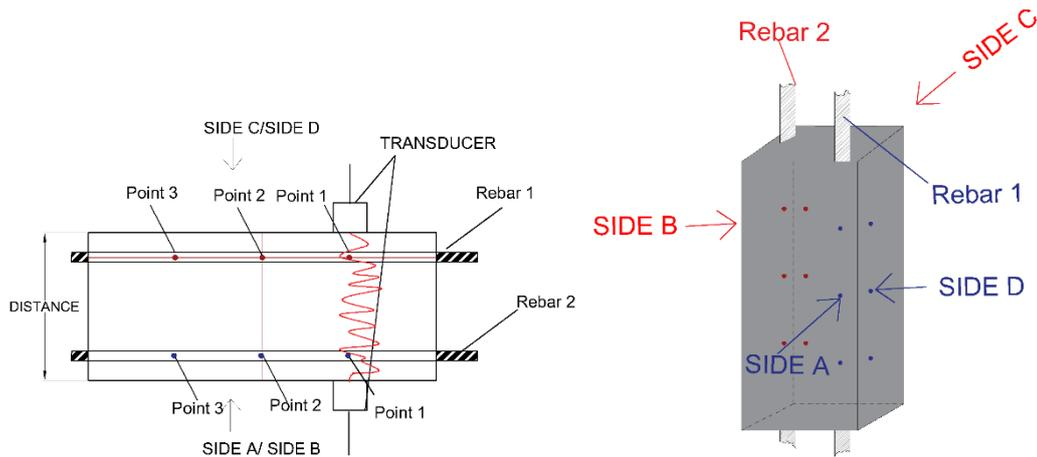
**Figure 5: Direct transmission measurement of UPV values of Specimen**
