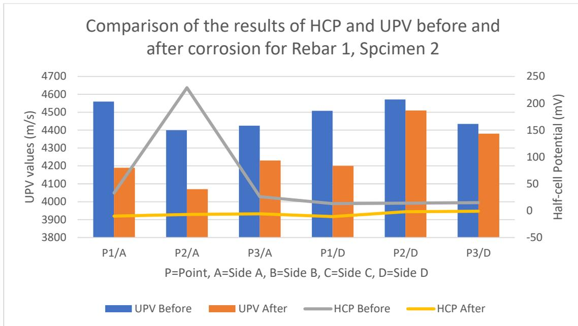
**Figure 11: The Comparison of the results of HCP and UPV before and after corrosion for Rebar1, Specimen 2**
