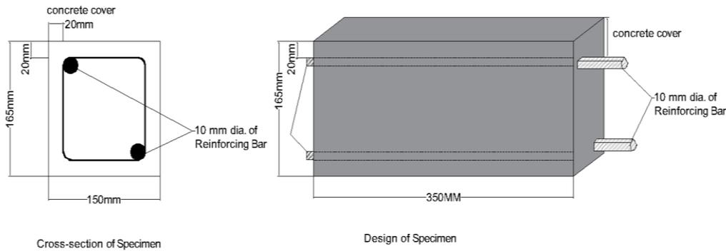
**Figure 3: Details of Specimens**
