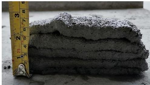
**Figure 4: Measurement of printed layers**
