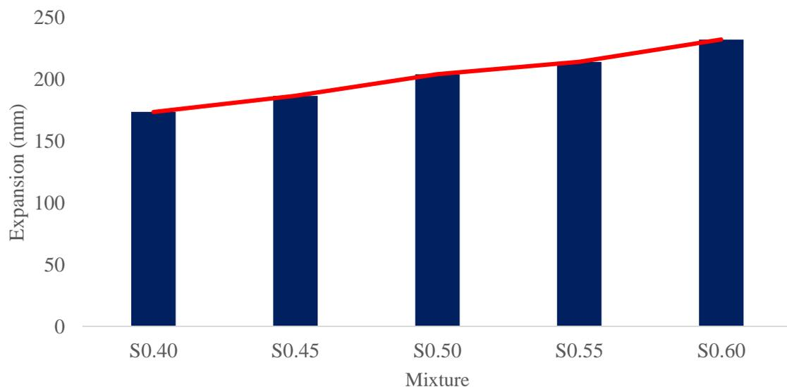
**Figure 5: Flow table reading versus difference w/c ratio mixture.**
