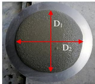
**Figure 2: Dimension of the measurement of the spread**
