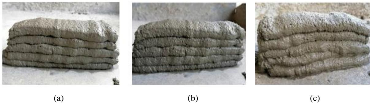
**Figure 7: (a) Buildability mixture 0.50, (b) Buildability mixture 0.55, (c) Buildability mixture 0.60.**
