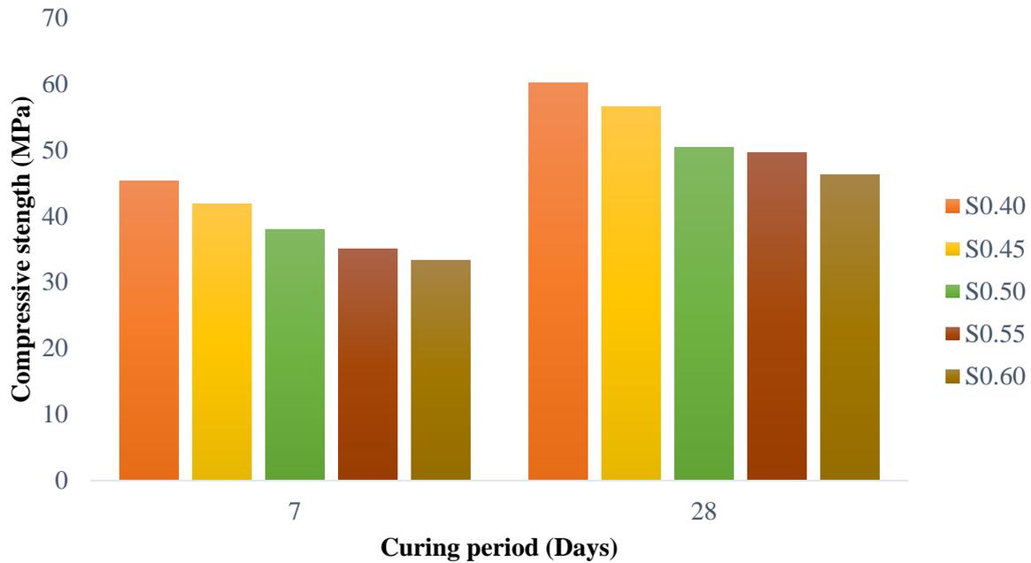
**Figure 8: Compressive strength of the concrete versus curing period.**
