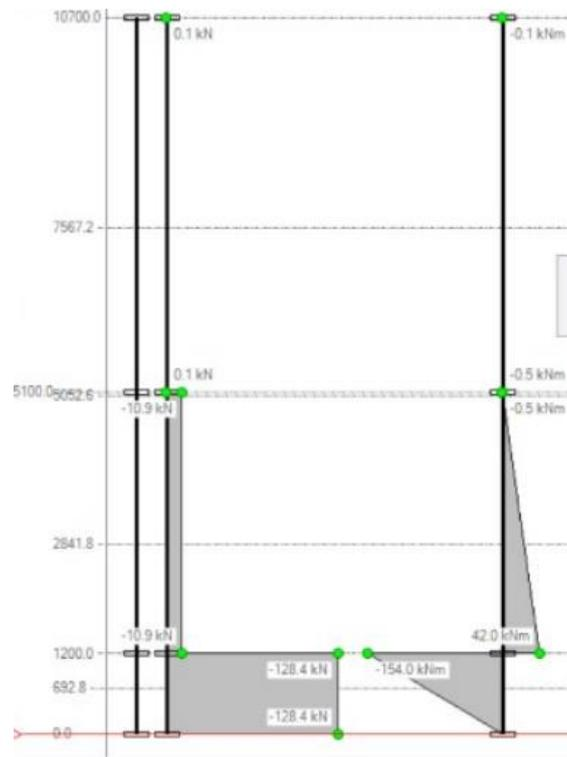
**Figure 6: Max SFD and BMD on Column**
