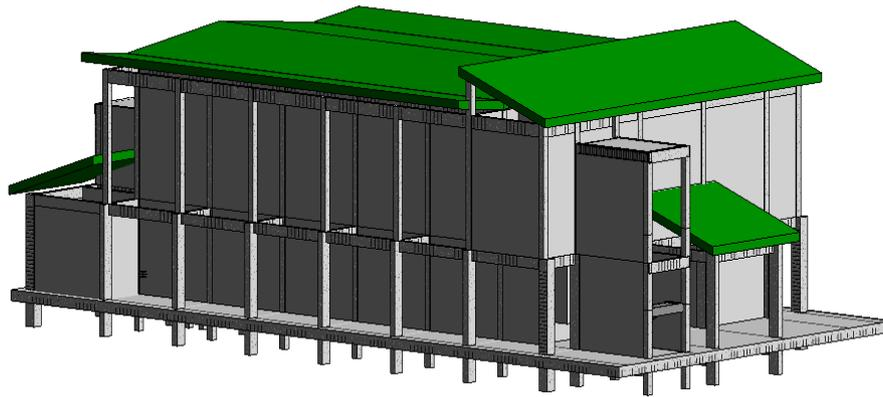
**Figure 12: Element brickwall and roof in Autodesk REVIT**
