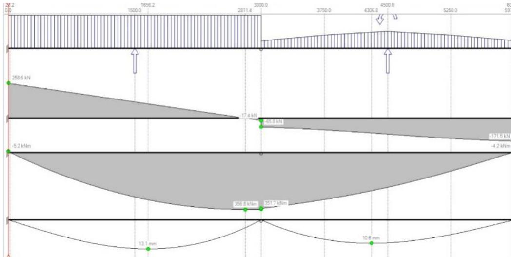
**Figure 5: Max SFD and BMD on Beam**
