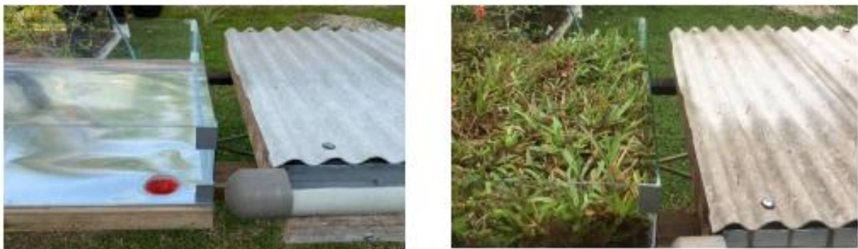
Figure 2. Green roof and Conventional roof model setup
