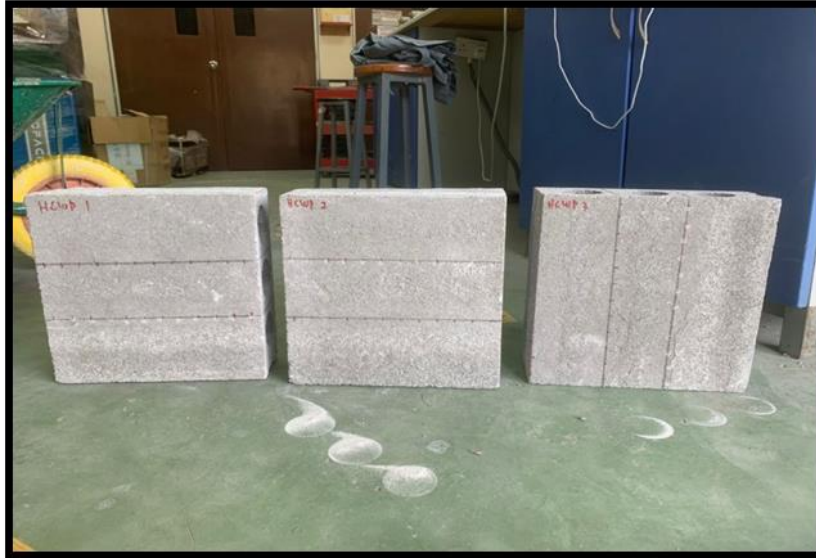
Figure 1: HCWP samples with dimension 300 mm x 300 mm x 100 mm
