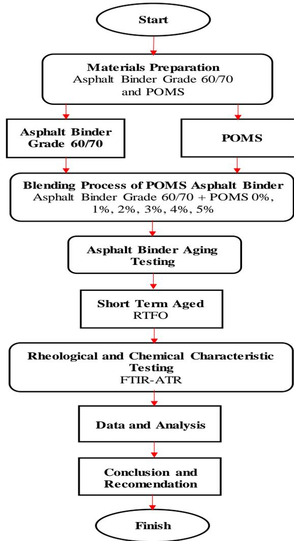
**Figure 1: Flow process of the experiments**
