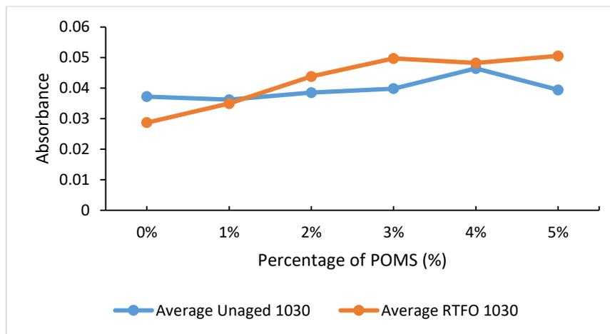
**Figure 6: Comparison of sulfoxide absorbance for unaged and STA POMS modified asphalt binder**
