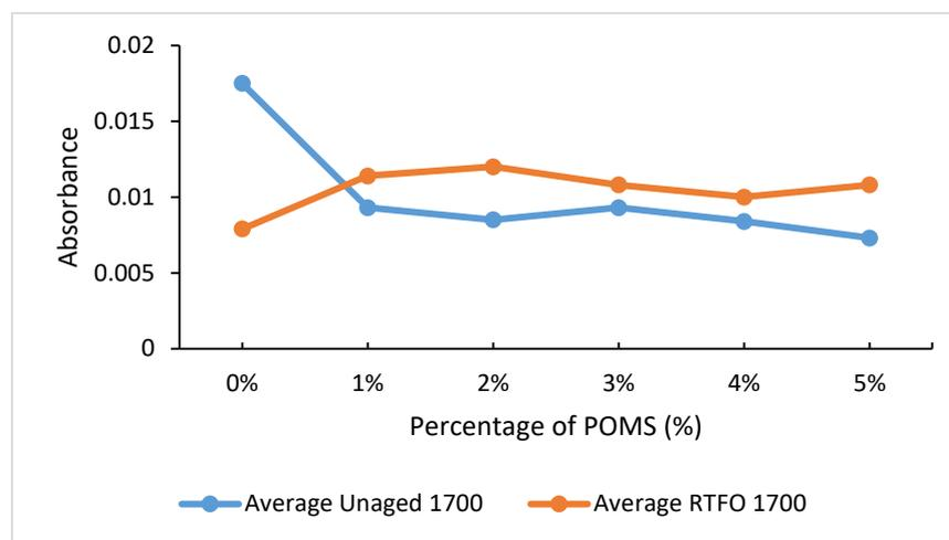
**Figure 7: Comparison of carbonyl absorbance for unaged and STA POMS modified asphalt binder**
