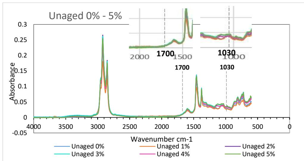
**Figure 4: FTIR absorbance spectra for carbonyl and sulfoxide group for unmodified and POMS modified asphalt binder (unaged)**
