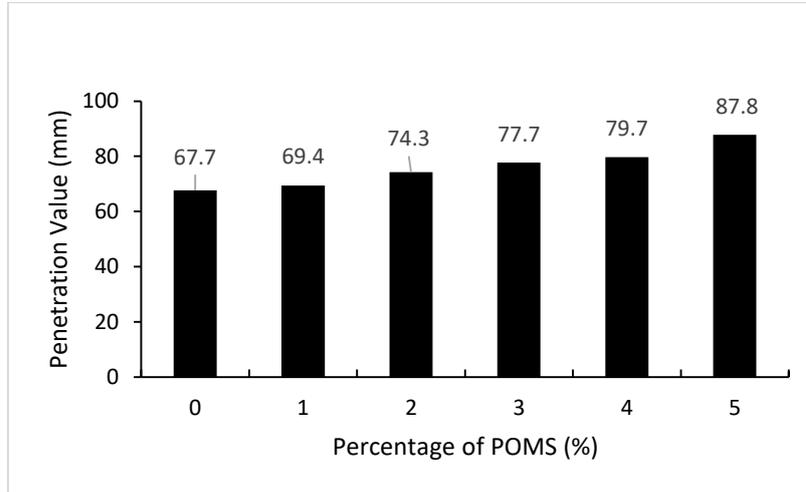
**Figure 2: Penetration value of unmodified and POMS modified asphalt binder.**
