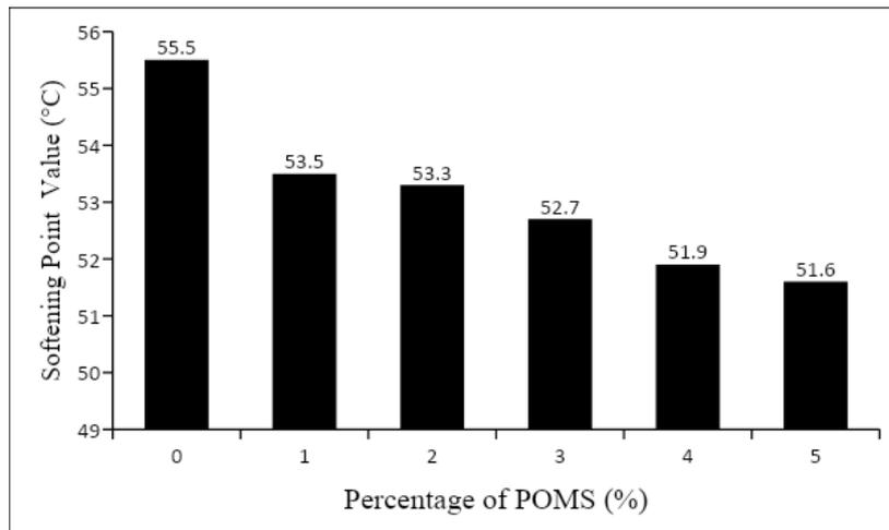
**Figure 3: Softening point of unmodified and POMS modified asphalt binder**
