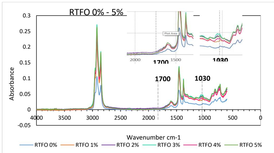
**Figure 5: FTIR absorbance spectra for carbonyl and sulfoxide group for unmodified and POMS modified asphalt binder (unaged)**
