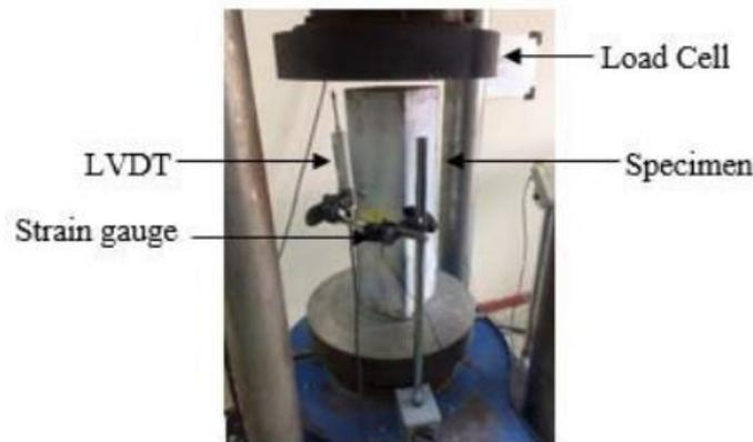
Figure 1: Test Specimen Set Up [9]
