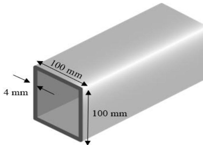
**Figure 2: Dimensions of the hollow section [9]**
