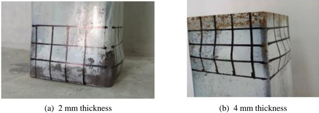
**Figure 4: Failure mode of the 2 mm and 4 mm steel fibre foamed CFHS specimens [9]**
