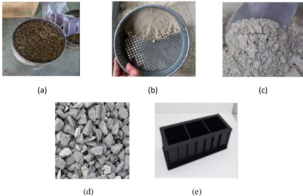
Figure 1 - Materials use for pumice LWAC: (a) pumice aggregate, (b) fine aggregate, (c) Ordinary Portland Cement, (d) coarse aggregate, (e) concrete mould
