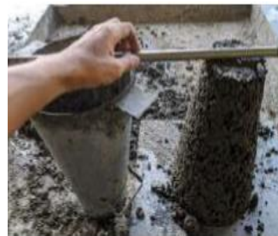
Figure 3: Measuring the slump
