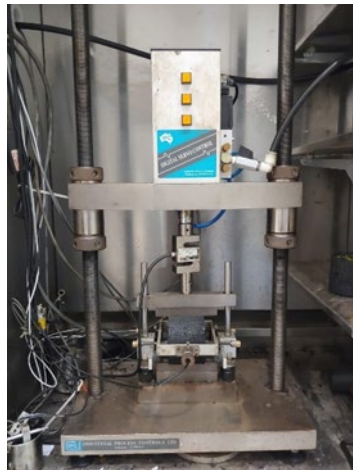
Figure 3.1: Indirect tensile fatigue test on UTM
