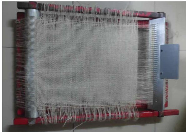
Figure 1: The weaving of kenaf yarn using handloom machine
