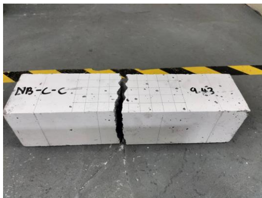
(a) Beam fracture
