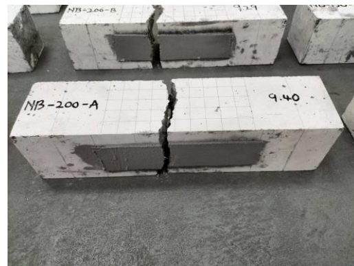
(b) KFRP fracture
