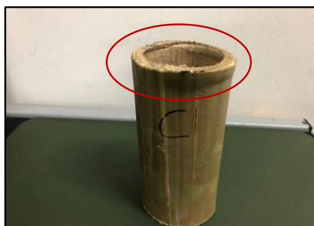
Figure 9: Bamboo C after CS test has done, end bearing failure observed (in red)
