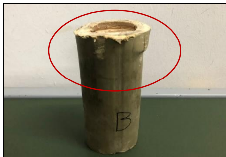
Figure 8: Bamboo B after CS test has done, end bearing failure observed (in red)
