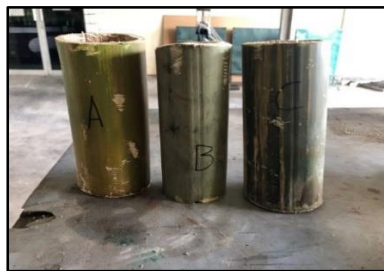
Figure 1: Bamboo samples A, B and C (all samples were cut with height, h = 150 mm)
