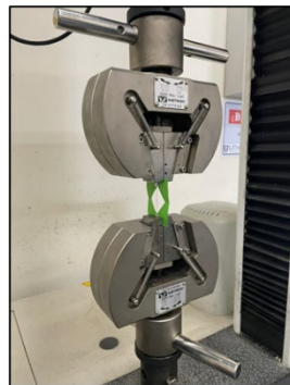
Figure 1: Instron Universal Testing Machine (ASTM D3379)
