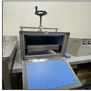
Figure 2: Solteq model HE110(Guarded Hot Plate)
