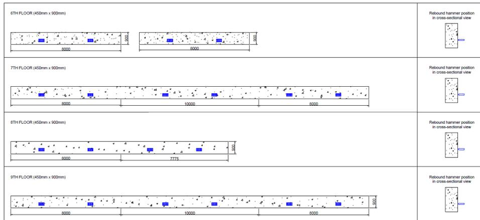
**Figure 2: Schematic diagram of rebound hammer test points on beam structures**
