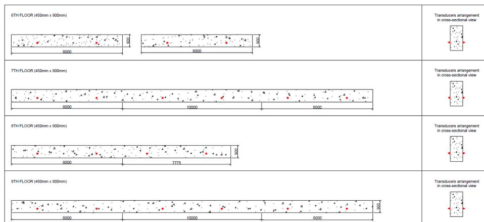
**Figure 3: Schematic diagram of Ultrasonic Pulse Velocity test points on beam structures**
