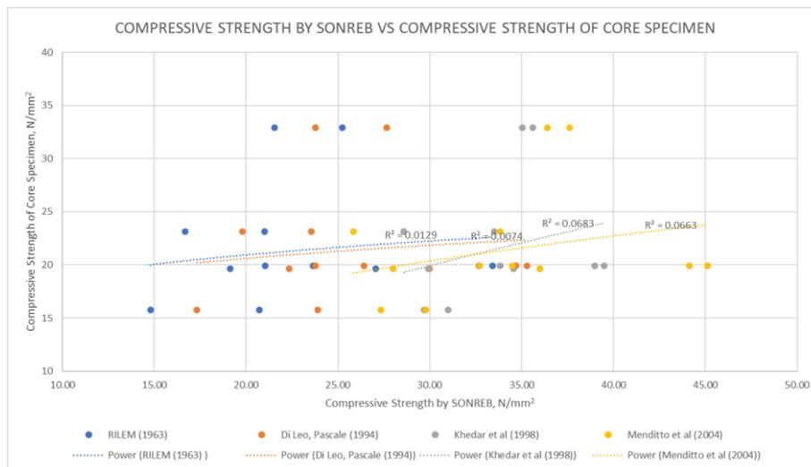
Figure 5: Compressive strength by SONREB vs compressive strength of core specimen
