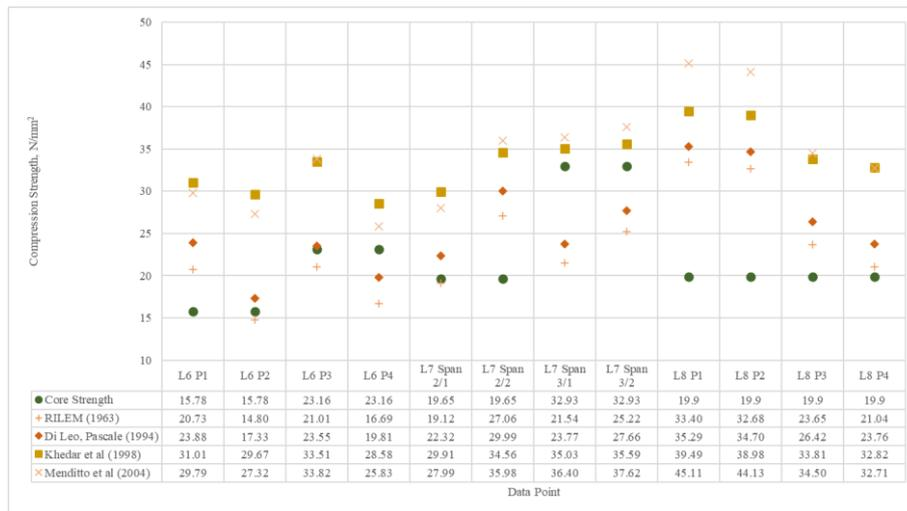
Figure 4: Comparison between core strength and compressive strength by SONREB conversion
