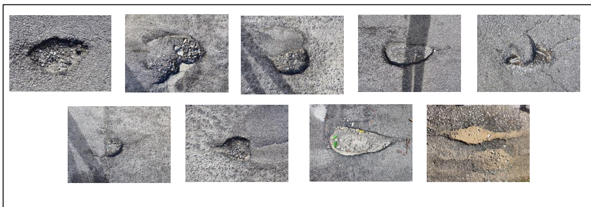
Figure 8: Final report for the potholes assessment through Mobile Potholes Interpreter
