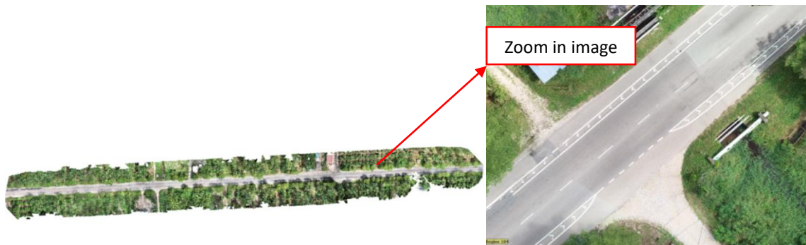
Figure 3: Orthomosaic Images Produced using Pix4DMapper
