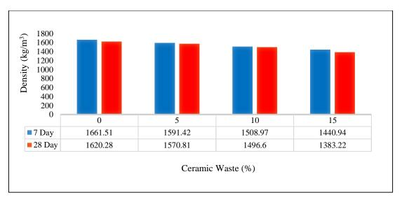
Figure 3: Relationship between density and percentage of ceramic waste
