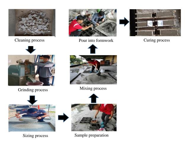
Figure 1 : Flow chart of fabricating process of CWB
