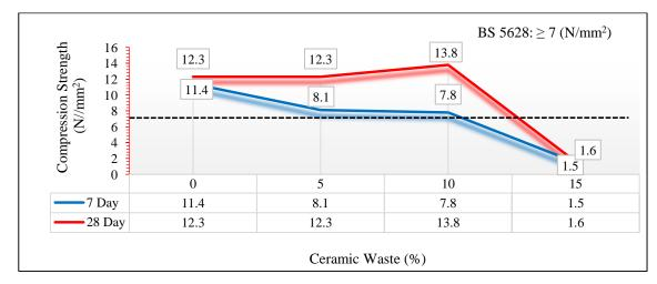
Figure 5: Compressive strength of the samples according to the percentage of ceramic waste for 7 and 28 days of curing
