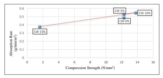
Figure 11: Relationship between compressive strength and absorption for 28 days
