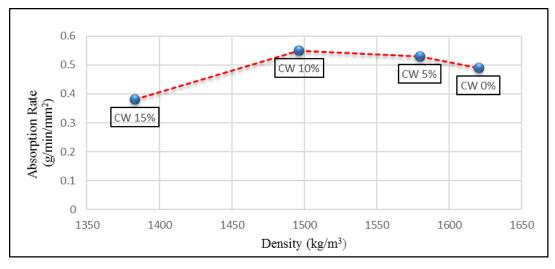
Figure 9: Relationship between the density and absorption for 28 day
