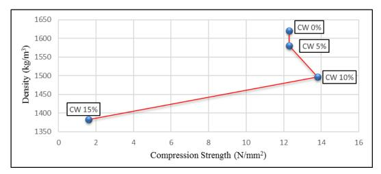
Figure 7: Relationship between compressive strength and density for 28 days
