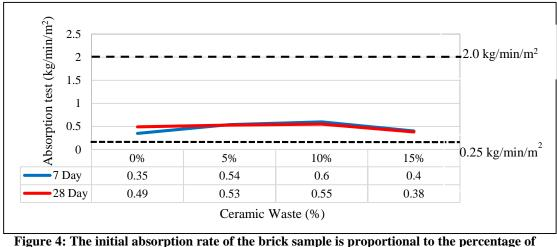
al absorption rate of the brick sample is proportional to th
