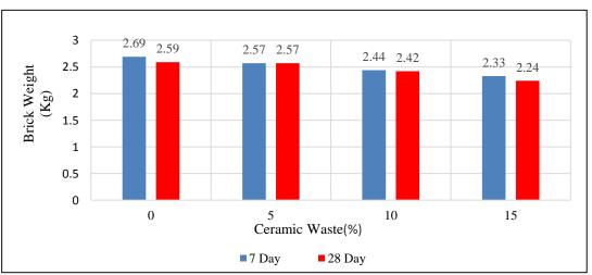
Figure 2: Relationship between brick sample weight to ceramic waste percentage
