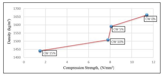
Figure 6: Relationship between compressive strength and density for 7 days
