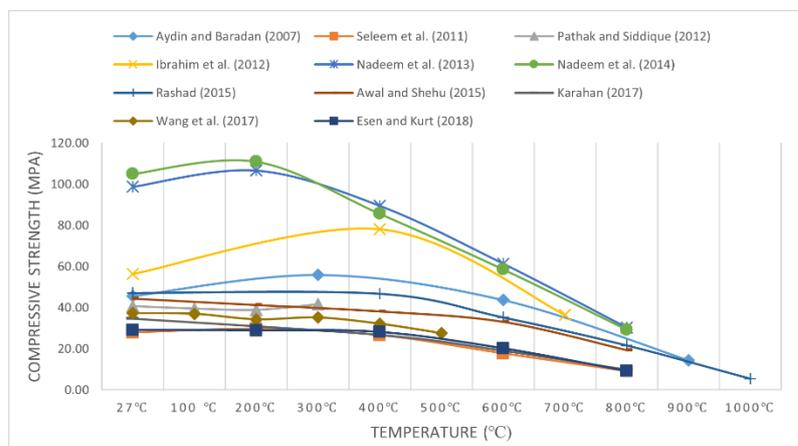
Figure 1: Compressive Strength of FA Control Sample
