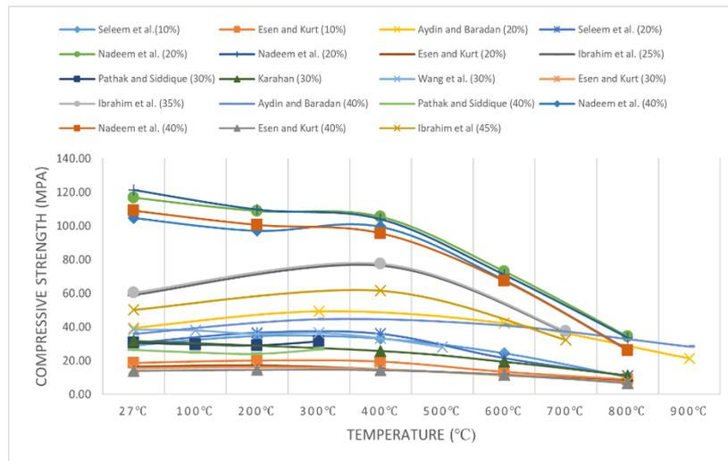
**Figure 2: Compressive Strength of 10% to 40% FA Replacement**
