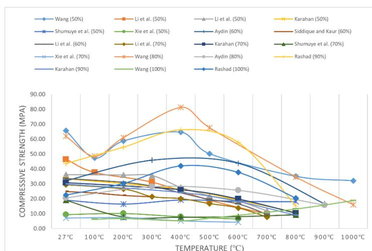
**Figure 6: Compressive Strength of 50% to 100% of GGBS Replacement**
