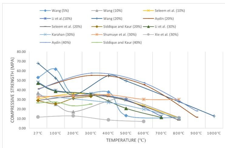
**Figure 5: Compressive Strength of 5% to 40% GGBS Replacement**
