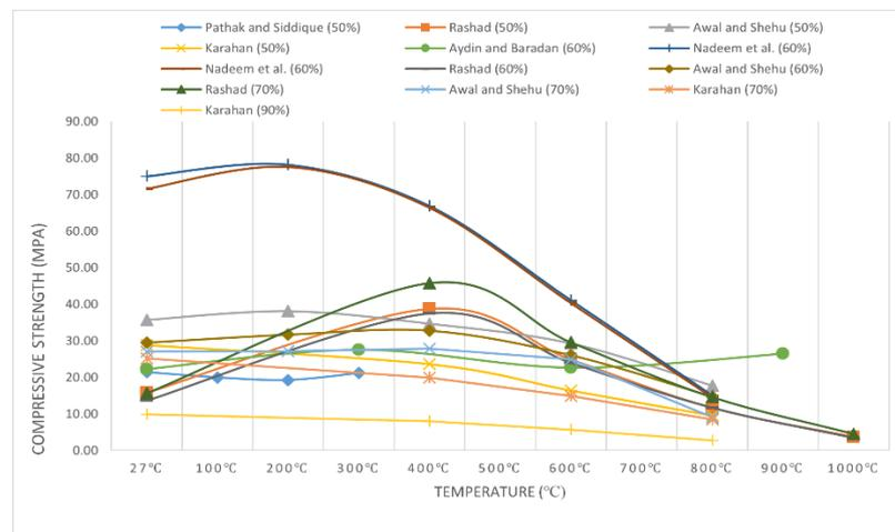
**Figure 3: Compressive Strength of 50% to 90% FA Replacement**
