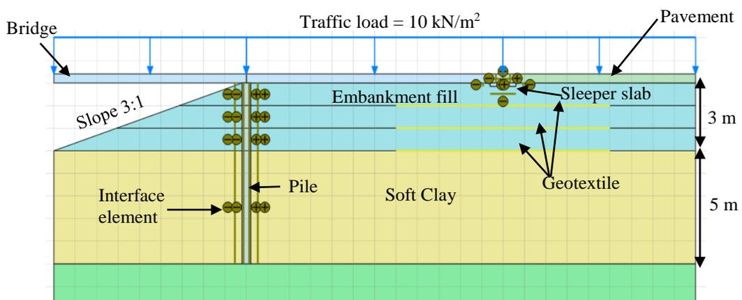
Figure 5: Model for triple layers of geotextile
