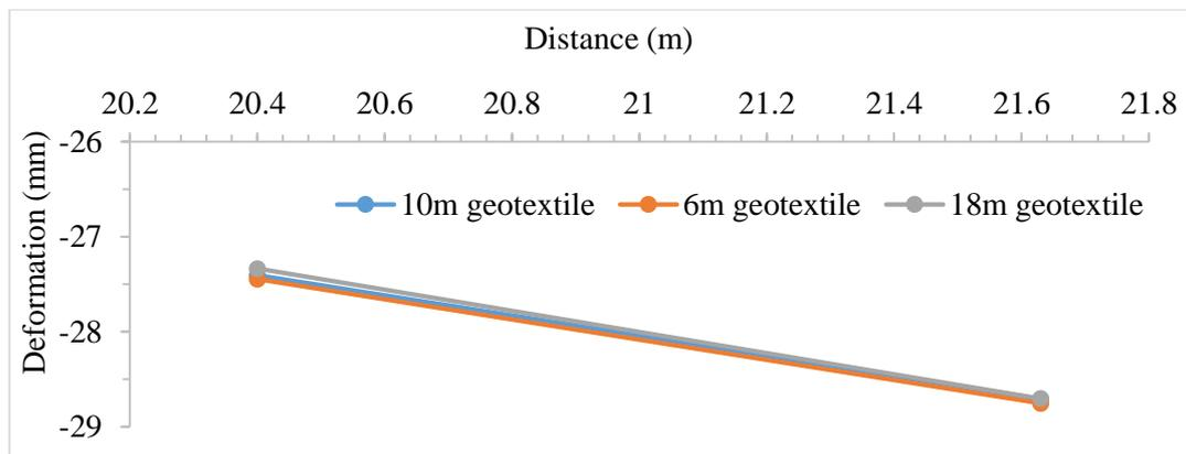
Figure 9: Vertical displacement of different geotextiles length
