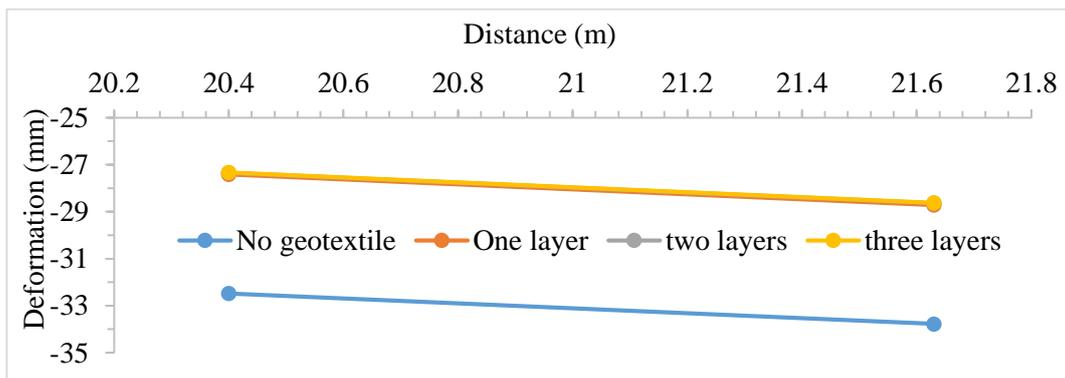
Figure 8: Vertical displacement of different geotextiles layer
