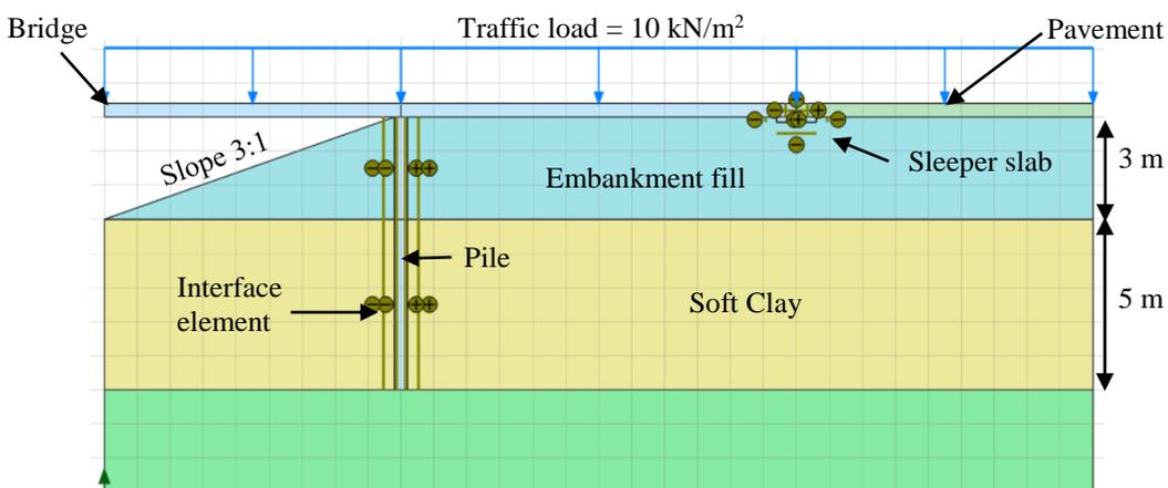
Figure 2: Model for unreinforced approach slab
