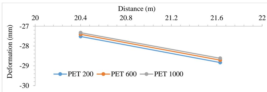
Figure 10: Vertical displacement of different geotextiles stiffness
