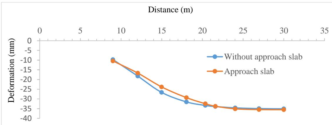
Figure 7: Deformation-distance in the model with and without approach slab
