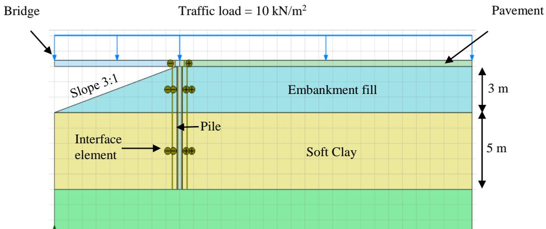
Figure 1: Model for unreinforced pavement
