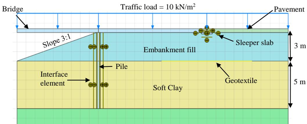
Figure 3: Model for a single layer of geotextile
