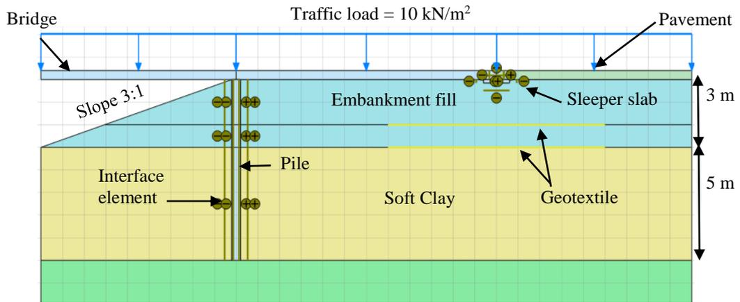
Figure 4: Model for double layers of geotextile
