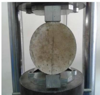
Figure 3: Split tensile strength test
