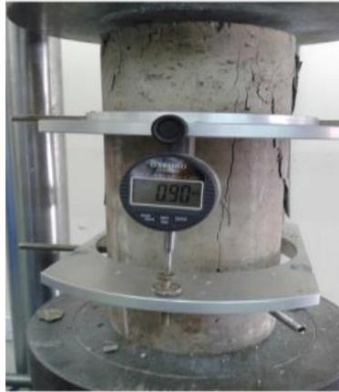
**Figure 4: Modulus of elasticity test**
