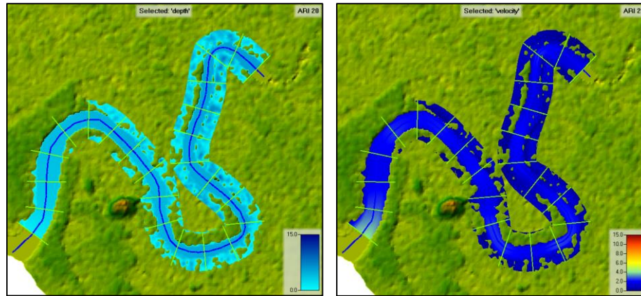
Figure 11: Depth and Velocity map of the flow for ARI 20 years
