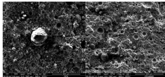
**Figure 2: The microstructure of coal FA geopolymer cured at room temperature and elevated temperature respectively [8]**
