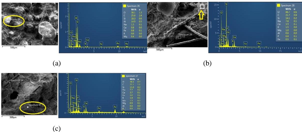
Figure 5: The SEM micrograph of geopolymer added with specific content. (a) superplasticizer and water. (b) water. (c) superplasticizer [15]
