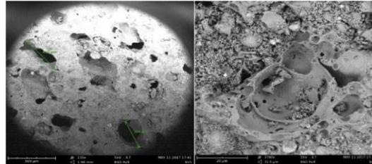
Figure 4: The SEM micrographs of geopolymer foam with the magnification of 137x and 3700x respectively [13]
