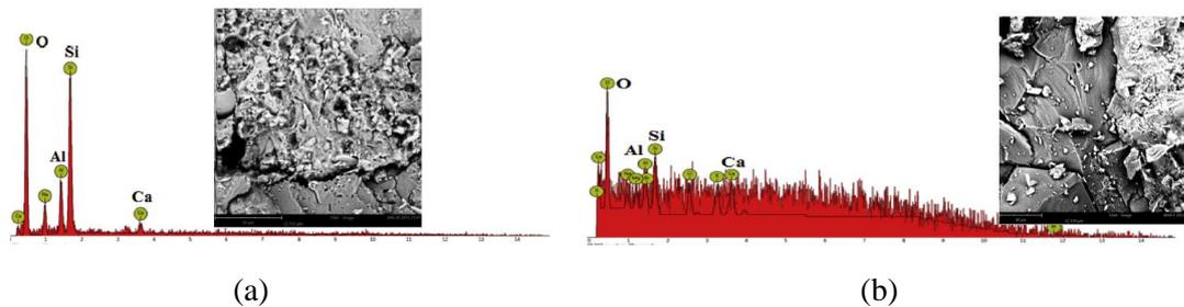
**Figure 6: The SEM and EDS micrograph of POFA geopolymer concrete with specific content. (a) 100% of palm oil clinker coarse aggregate. (b) 50% of palm oil clinker and 50% of oil palm shell as the coarse aggregate.**
