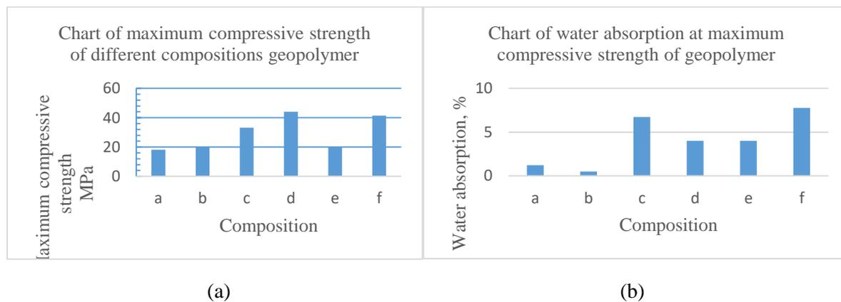
**Figure 7(a) Maximum compressive strength of different compositions geopolymer, (b) Water absorption at maximum compressive strength of geopolymer**
