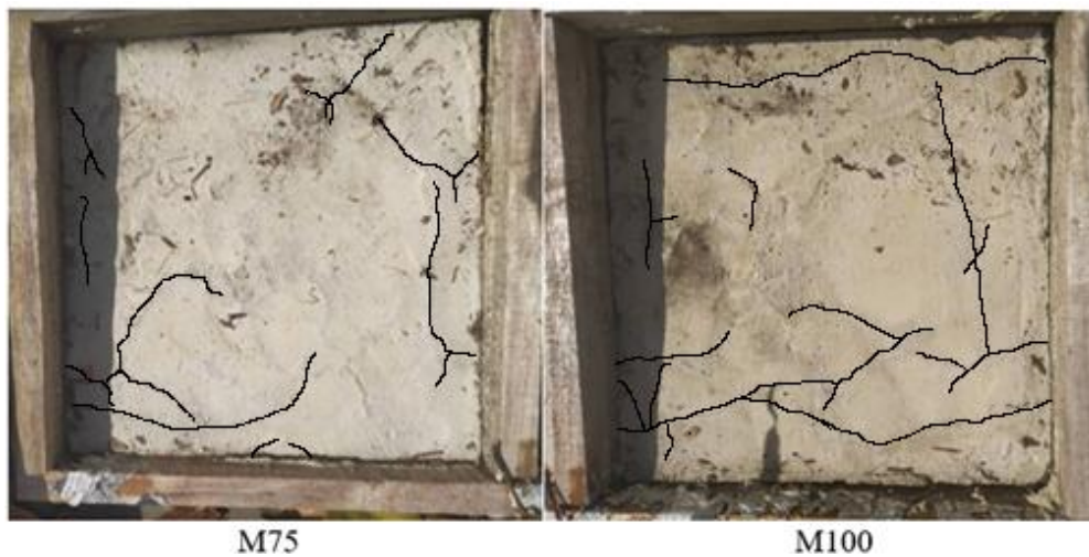
Figure 18: Uncured panel specimens for M75 and M100 at 60 th day
