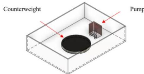
Figure 2: Isometric View of Buoyancy Control Device
