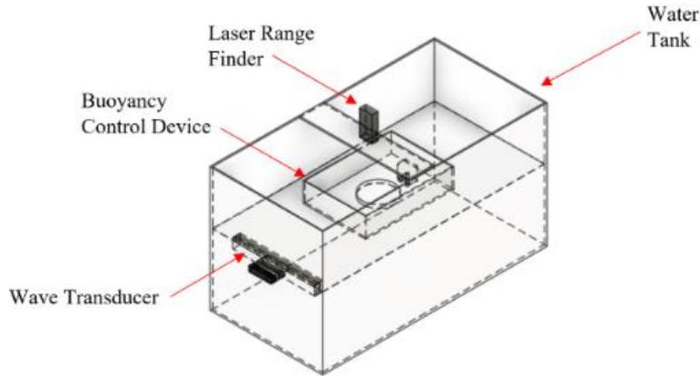
**Figure 6: Isometric View of Experimental Setup**
