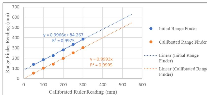
**Figure 7: Linearity and Bias of Laser Range Finder Benchmarked against Calibrated Rule**
