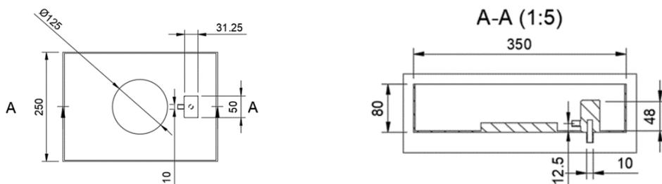
Figure 3: Cross sectional (left) and Top (right) View of Buoyancy Control Device
