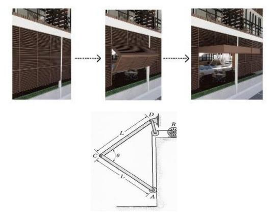
Figure 8: The Working Mechanisme of Adjustable Folding Aluminium Louvres
