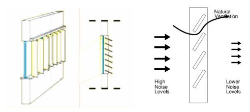
Figure 7: Louvres allowing natural air flow while reducing the noise impact
