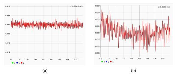
Figure 8: Vibration velocity on 29th November 2020 at 9 am (a) 2 m (b) 8 m
