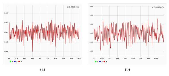
Figure 9: Vibration velocity on 29th November 2020 at 2 pm (a) 2 m (b) 8 m
