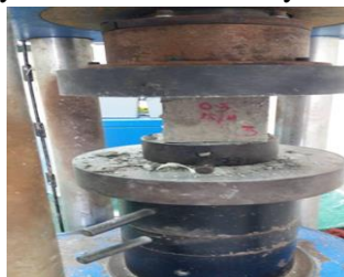
Figure 5: Compressive strength test
