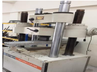
Figure 6: Flexural strenght test
