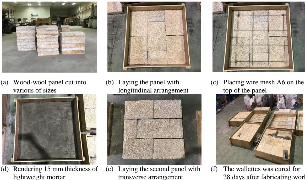
**Figure 3: Fabrication process of wallets**
