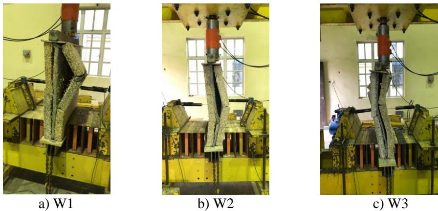
**Figure 7: Failure mode of wallettes**
