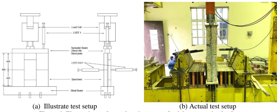
**Figure 4: Illustration and actual testing setup of axial compression load**
