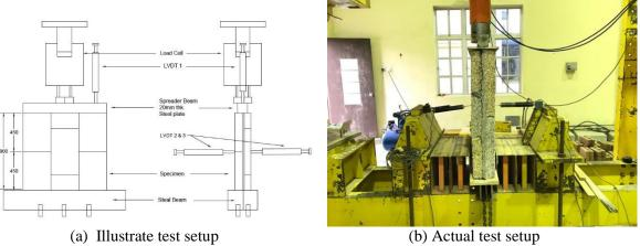
Figure 4: Illustration and actual testing setup of axial compression load
