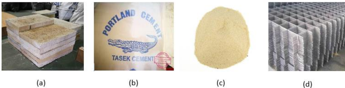
Figure 1: (a) WWCP (b) Portland cement (c) fine sand (d) A6 wire mesh
