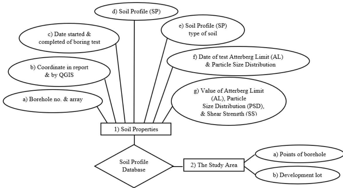
**Figure 3: ER-Diagram entity relationship diagram**
