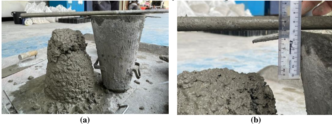
Fig. 1 (a) Slump test conducted on concrete mix sample; (b) Slump value observed from the concrete mix sample
