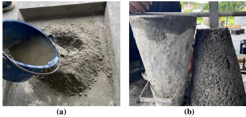
Fig. 2 (a) Batching concrete; (b) Slump test
