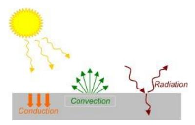
Figure 2: Heat transfer process in pavement layer [7]
