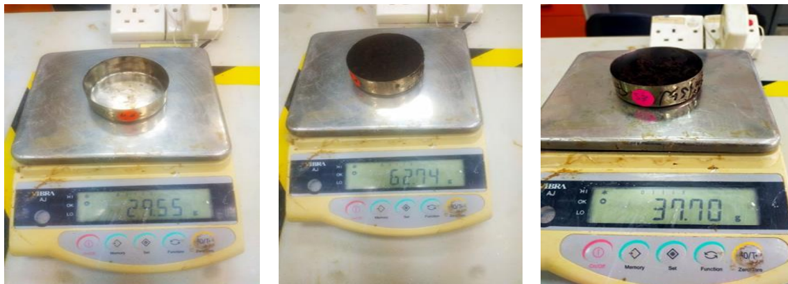
Fig. 3 Process Obtain Moisture Content Data of Peat Soil Sample
