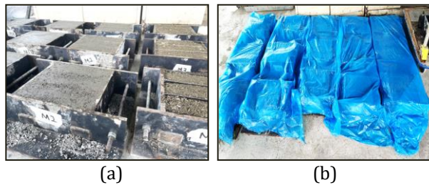
Fig 5 Process demould and curing (a) Labelled sample; (b) Labelled and demoulded
