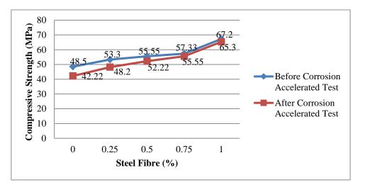
Figure 2: Comparison of compressive strength before and after conducting accelerated corrosion test [16]
