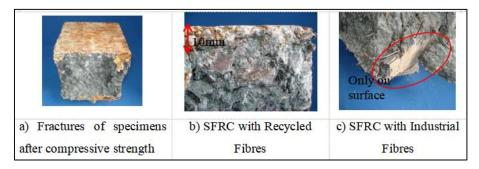
Figure 5: Internal analysis of specimens after 5 months of accelerated corrosion test [11]
