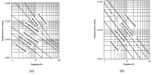
Figure 2: Design criteria based on acceleration limit (a) Reiher-Meister scale [54], (b) Modified **Reiher-Meister scale** [55]
