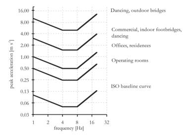
Figure 3: Limitation of acceptable acceleration levels for various usage of floors [58]
