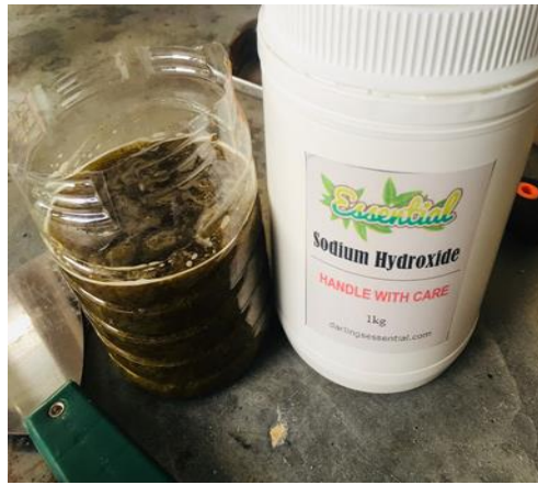
Figure 1: Submerging pineapple leaf fibers in naoh solution
