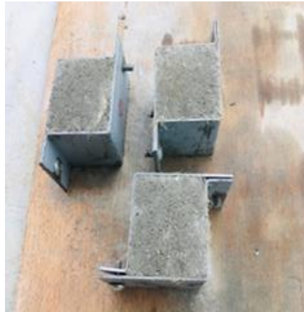
Figure 2: Casting of cement brick in mould
