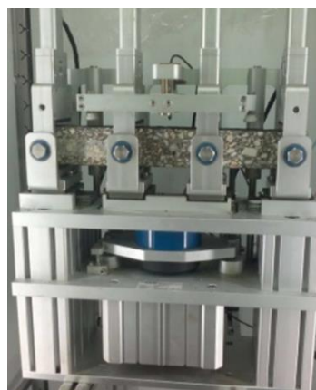
Figure 2: Close-up of beam with 4 clamps in place [5]
