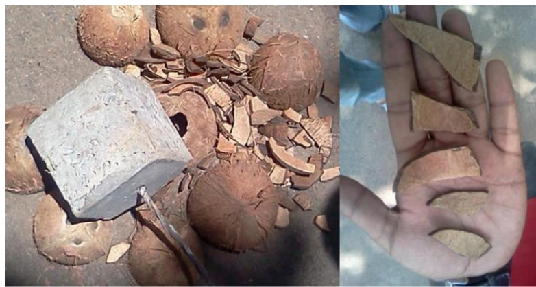
Figure 1: Transform coconut shell into aggregate
