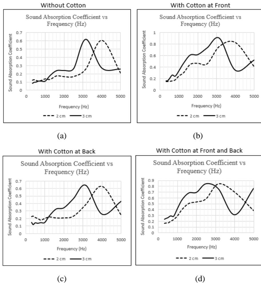
**Figure 6: Sound absorption coefficient of cotton bud sticks in (a) without cotton, (b) with cotton layer at front, (c) with cotton layer at back, (d) with cotton layer at front and back**
