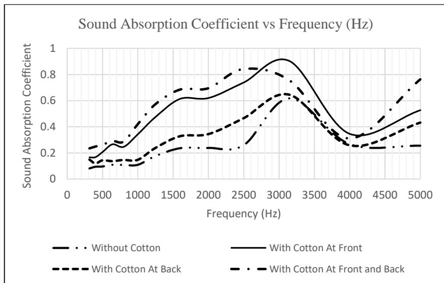
Figure 5: Sound absorption performance of sample with 3 cm thickness in four condition
