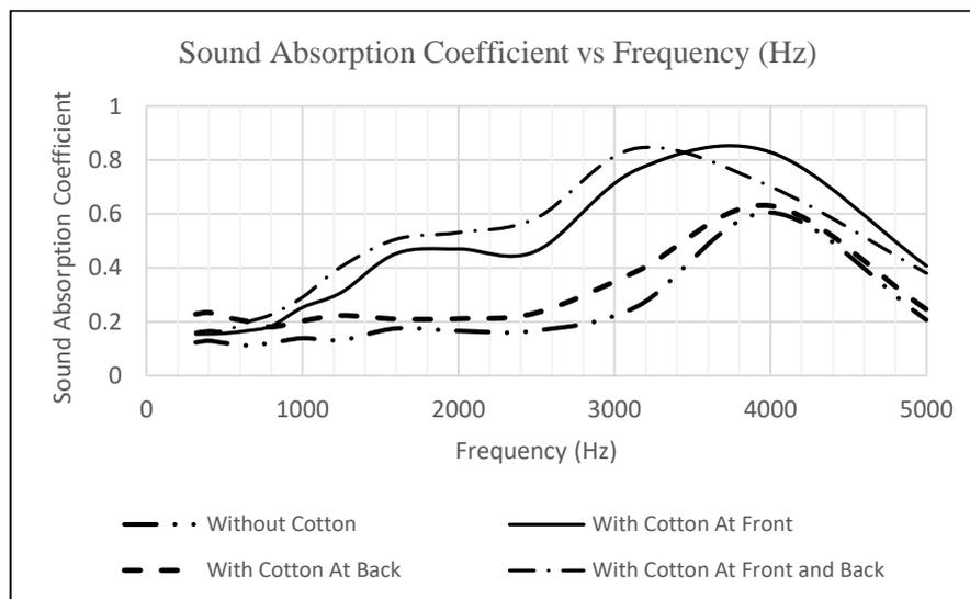
Figure 5: Sound absorption performance of sample with 2 cm thickness in four condition
