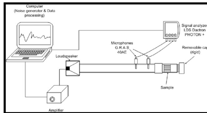
**Figure 4: Schematic diagram of experimental set-up**
