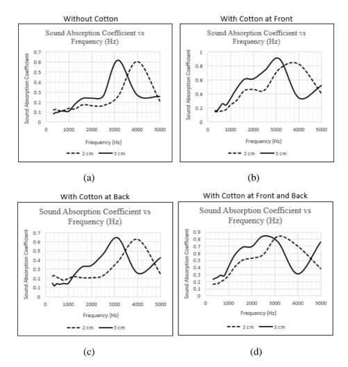
Figure 6: Sound absorption coefficient of cotton bud sticks in (a) without cotton, (b) with cotton layer at front, (c) with cotton layer at back, (d) with cotton layer at front and back
