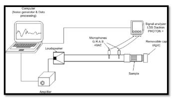
Figure 4: Schematic diagram of experimental set-up
