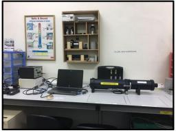
Figure 3: Impedance tube
