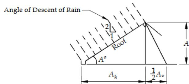
**Figure 2 Single slope roofing freely exposed to the wind (NAHRIM 2014)**
