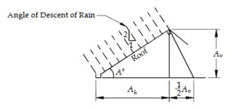
Figure 2 Single slope roofing freely exposed to the wind (NAHRIM 2014)
