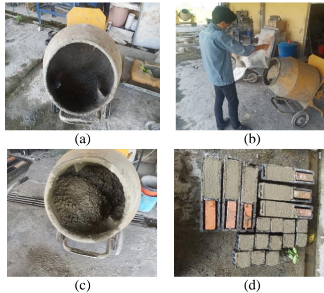
Figure 3: Mixing process: (a) The mixer has been filled with part of the water, (b) Materials have been added to the mixer, (c) Materials have been mixed for a period of time, (d) Pour the concrete into mould.
