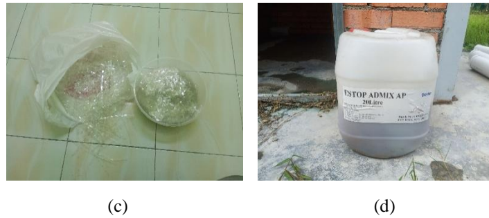
Figure 1: Preparation of materials: (a) Coarse Aggregates, (b) Fine Aggregates, (c) PET fiber (d) Superplasticizer
