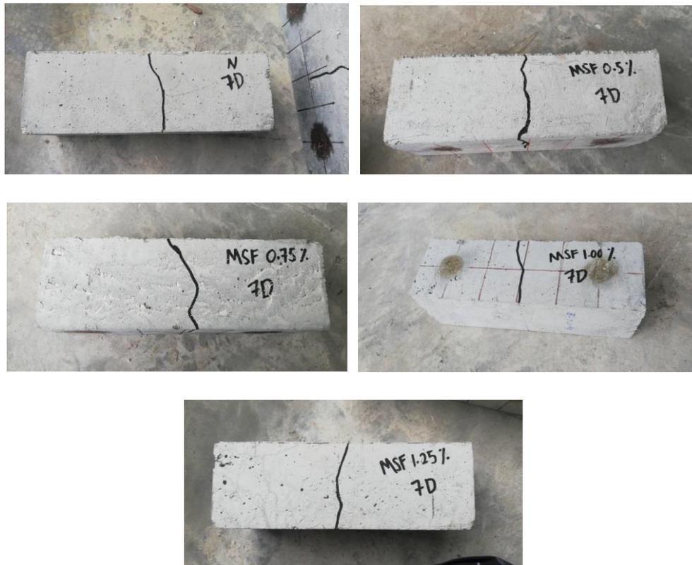
**Figure 5: 0%, 0.5%, 0.75%, 1.00%, and 1.25% of MSF concrete**
