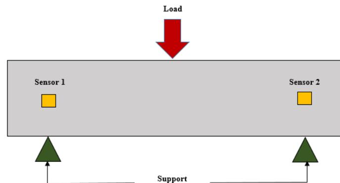
**Figure 1: Setup of Acoustic Emission (AE) sensors**
