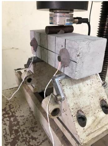
**Figure 2: Setup of AE test**
