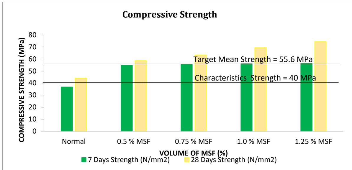
Figure 4: Compressive strength of concrete mix at 7 days and 28 days
