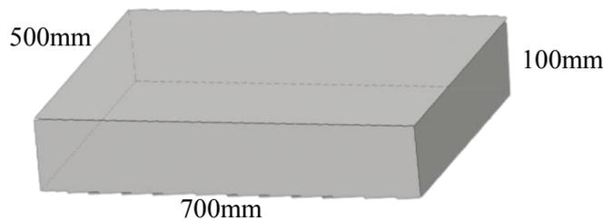
**Figure 1: Dimension of panel**
