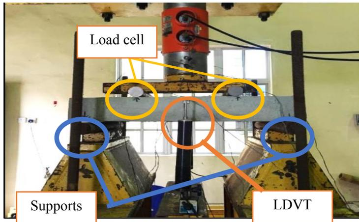
Figure 2: Four point bending test apparatus
