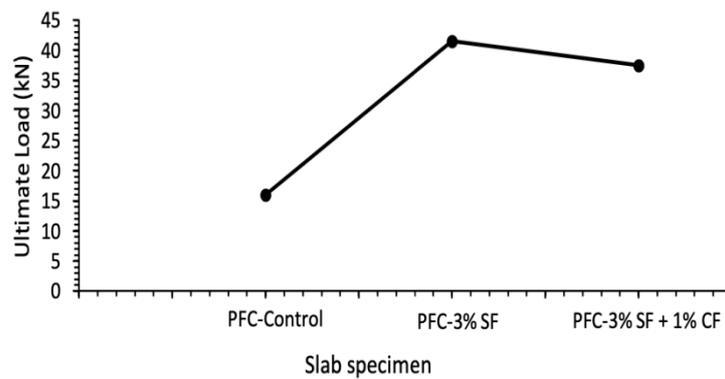
**Figure 4: Ultimate load of PFC for control, 3% SF and 3% SF + 1% CF**
