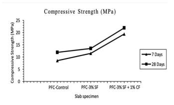
Figure 3: Compressive strength of specimen
