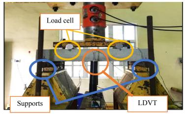
Figure 2:Four point bending test apparatus
