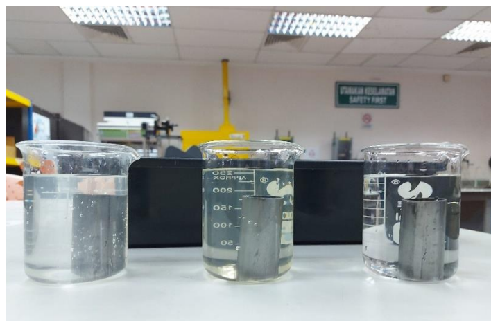
Figure 1: Immersion corrosion test set-up with piping and water samples
