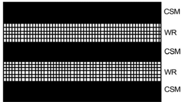
Figure 1: Layers of composite structure
