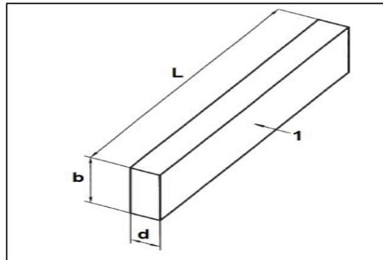
**Figure 3: Flatwise Charpy impact test**
