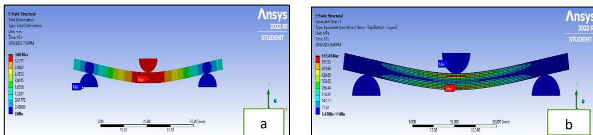
Figure 9: (a) deformation (b) equivalent stress
