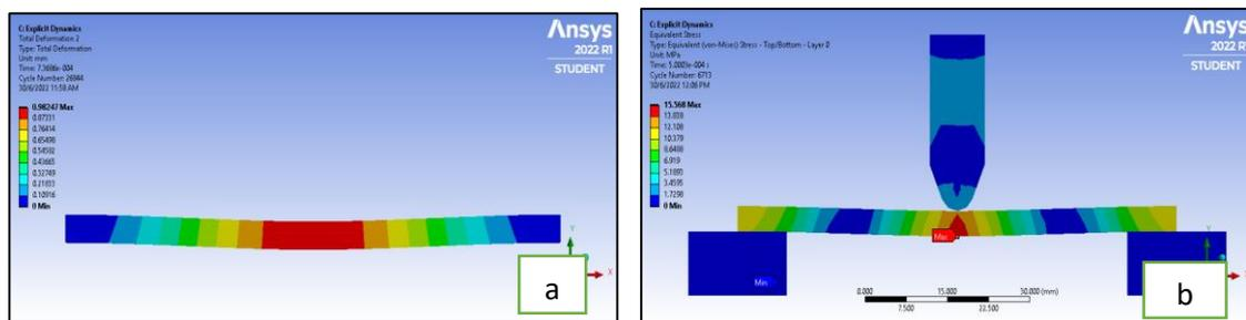
Figure 6 : (a) total deformation (b) Equivalent stress
