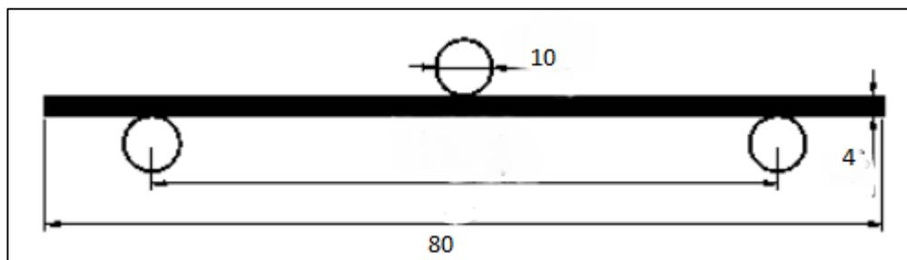
**Figure 4: Three-point bending setup**
